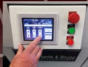
PLC / Intuitive Operator Interface
