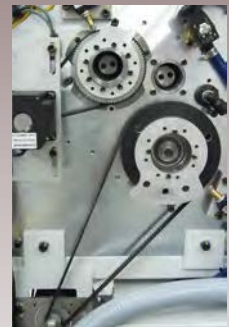
Automated Nip Adjustments via Stepper Motor & Eccentric Bearings
